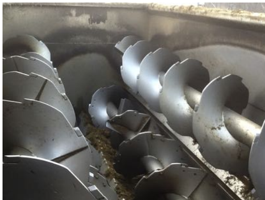
Fig. 10. TMRs under the augers indicate excessive wear, which decreases auger diameter and mixing ability.
