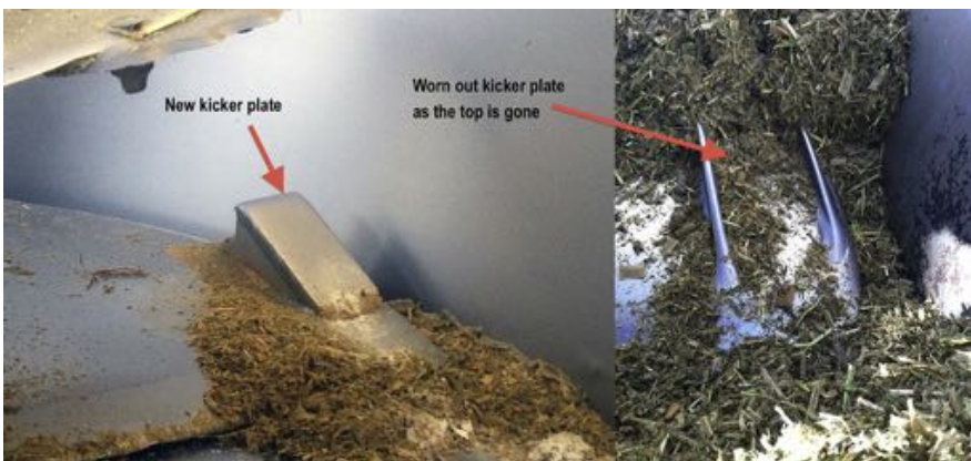
Fig. 14. A good conditioned (new) kicker plate (left photo) and a worn out kicker plate in Peecon vertical mixer boxes.
