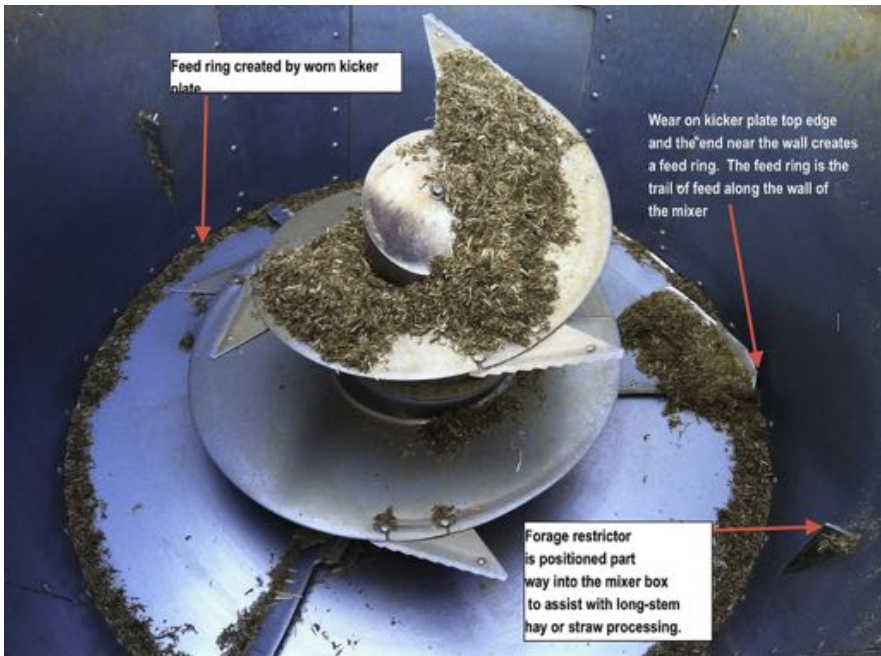
Fig. 12. TMR ring between augers and mixer wall suggests worn kicker plate and/or augers.
