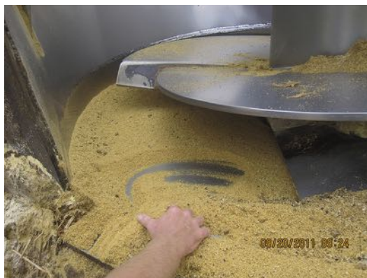
Fig. 15. The deflecting edge is worn off, allowing feed to build up on the floor of this Trioliet mixer box.
