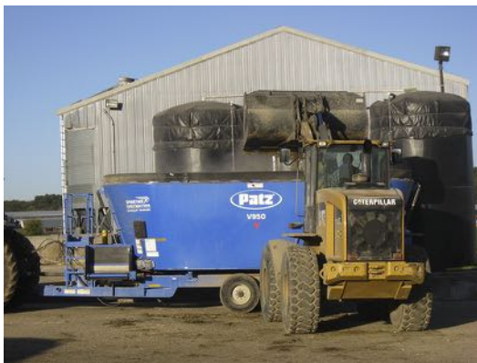
Fig. 20. Improper loading position on a dual-auger vertical mixer.
