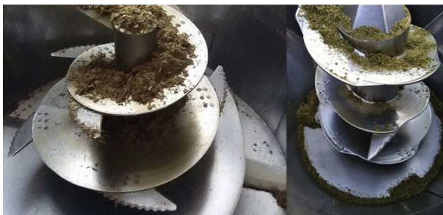
Fig. 16. Sharp knives in a vertical mixer box (left photo), and a vertical mixer with completely worn out knives (right photo).
